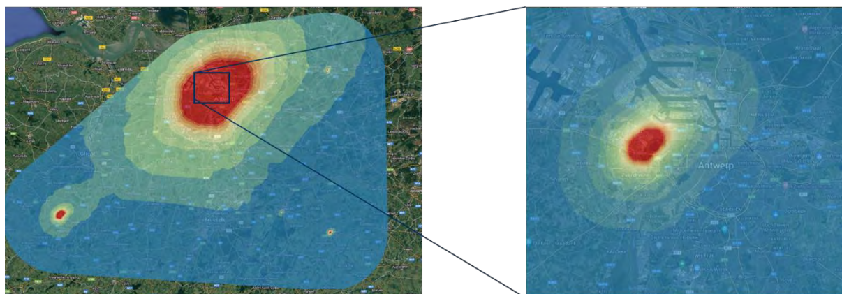
Figure 6. Left - PFK dispersion map for Flanders according to reported emissions. Right - detailed view of Antwerp
